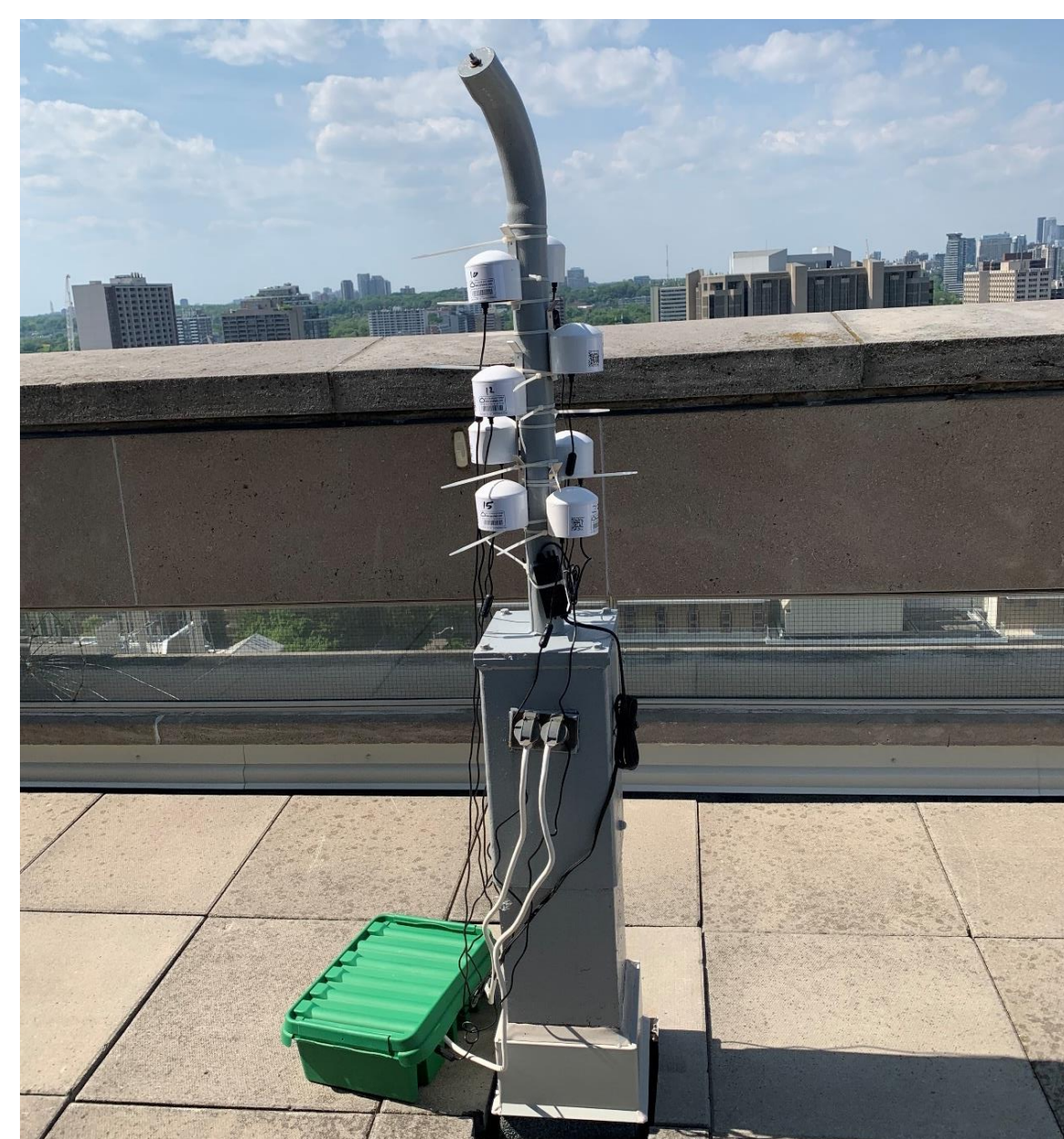
Figure 1: Ten of the PurpleAir sensors collocated on the roof of McLennan for calibration.
