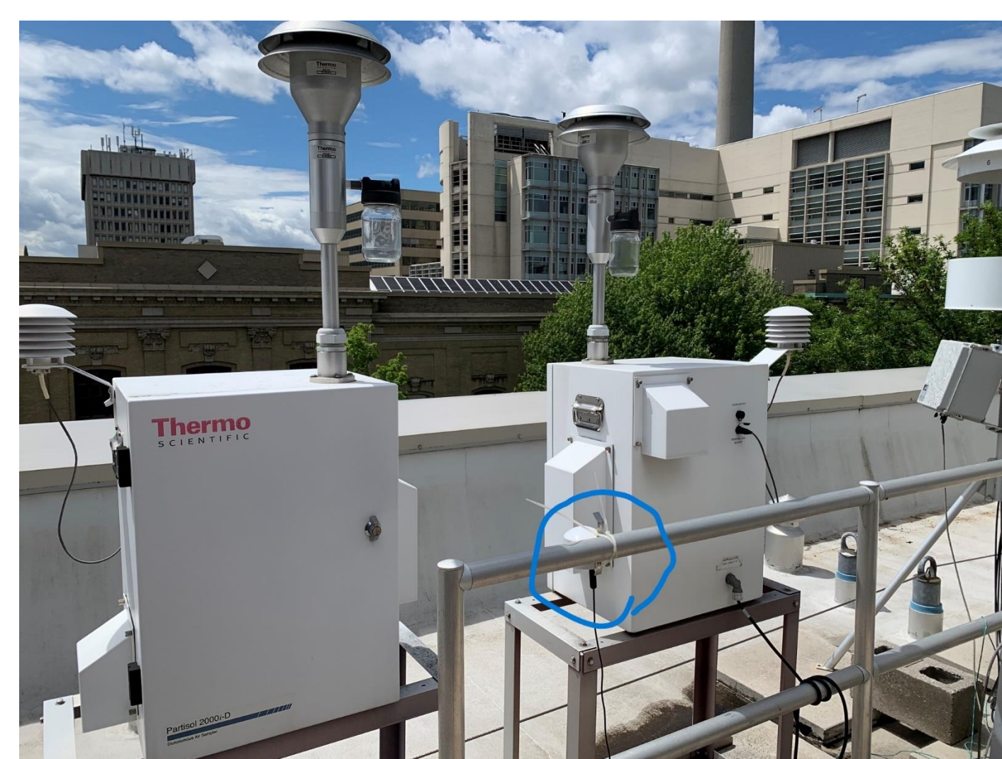
Figure 2: MP2 (circled in blue) collocated with the SHARP instrument on the Wallberg building.
